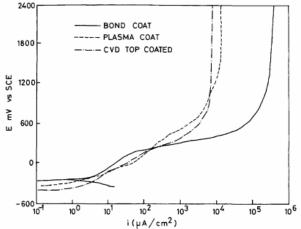
**Fig. 3.** Potentiodynamic polarization curves of (a) bondcoated substrate, (b) YSZ plasma sprayed onto bondcoated substrate and (c) CVD Zirconia on The plasmasprayed sample
