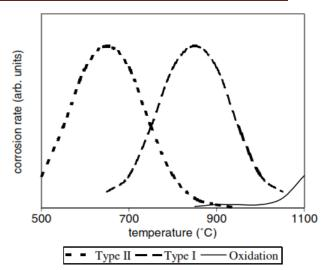
Fig.2 Schematic representation of rate-temperature curves for Type II hot corrosion, Type I hot corrosion andoxidation
